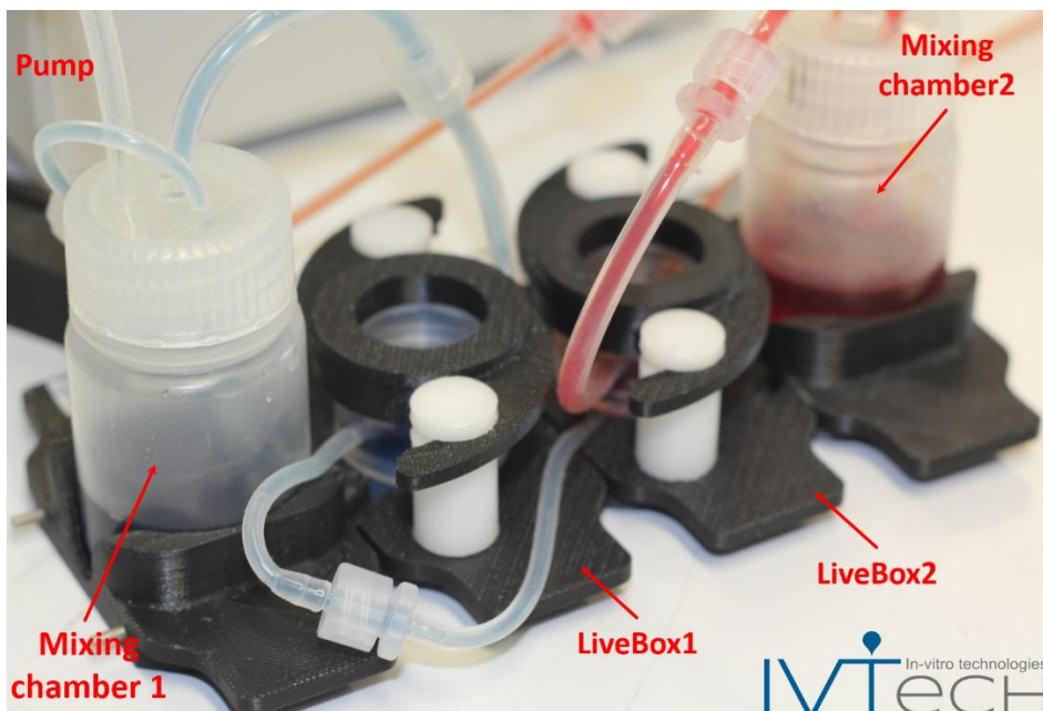
Figure 3. An example of a fluidic circuit composed by 2 mixing chambers, 1 LiveBox1, 1 LiveBox2, tubes and pump
